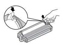
Turn the two levers on the toner cartridge with firm pressure.
